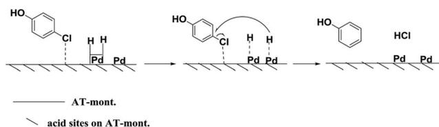
Scheme 1 A possible reaction pathway for the catalytic HDC of 4-CP on PdNP@AT-mont.
