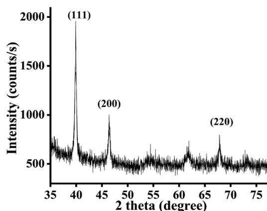
Fig. 3 PXRD spectra of PdNP@AT-mont. showing the different planes of Pd NPs.
