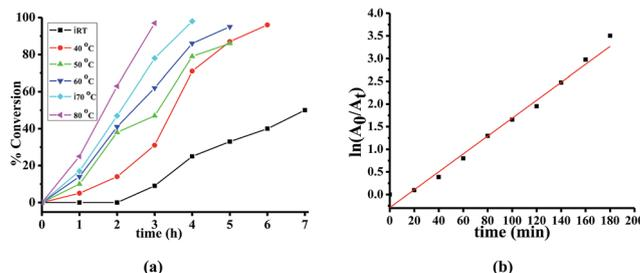
Fig. 7 (a) Pattern of progress HDC of 4-CP with time at different temperature and (b) the dynamics of HDC of 4-CP at 80 °C.
