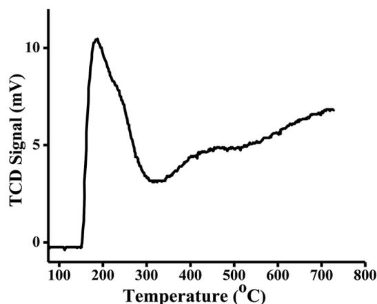
Fig. 2  $NH_3$ -TPD profile of AT-mont. indicating the presence of different types of acid sites on the surface.
