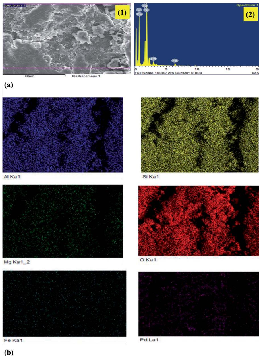
Fig. 4 (a) (1) SEM image and (2) EDX spectra of PdNP@AT-mont. (b) Elemental dot mapping of Al, Si, Mg, O, Fe and Pd on PdNP@AT-mont.
