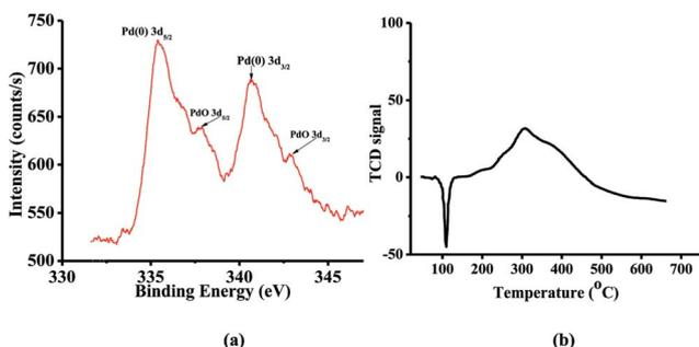
Fig. 6 (a) XPS spectra of PdNP@AT-mont. showing the presence of Pd(0) with formation of PdO and (b) H<sub>2</sub>-TPR of PdNP@AT-mont.
