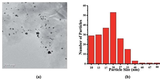
Fig. 5 (a) TEM image and (b) particle size distribution of PdNP@AT-mont.
